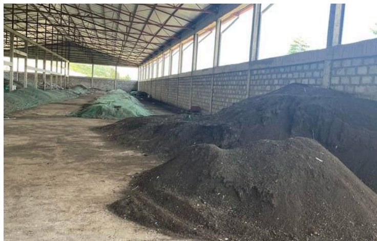
Compost curing under a roofed co-composting hall.
